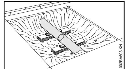
Support an exposed pipe in a trench so that it is stable and capable of bearing weight. If the ends of the pipe are firmly in the ground, the ground may act as a support where the pipe emerges into the open. Additional support will be needed closer to the cut, however, to prevent sagging (see illustration). Be alert for pipe that is under stress that may cause it to shift when cut; pipe in the ground may be under stress because of uneven pipe bed surfaces.
