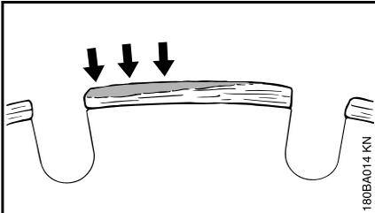
Built-up edges are identified by a pale grey deposit on the top of the diamond segments that clogs and blunts the segments.
