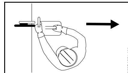
3. Position the cut-off machine in such a way that your body is clear of the cutting attachment. Avoid standing in direct line with the wheel (See illustration.) Never bend over the cutting attachment, especially when the guard is pulled back towards the top and there is a risk of reactive
