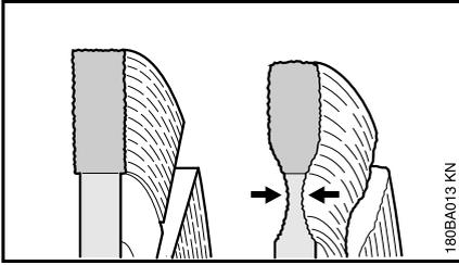
Undercutting is a wearing away of the steel core at or just below the diamond segments. When cutting road surfaces, do not cut through into the more abrasive ballast (gravel, crushed rock) below, as indicated by a light colored dust. This can cause excessive undercutting, resulting in wheel breakage and/or thrown segments.
