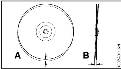
Excessive radial run-out (**A**) causes individual diamond segments to be overloaded and to overheat. This can in turn lead to stress cracking in the wheel core or to softening of individual segments.
