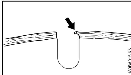
If you continue to use a cutting wheel with blunt segments, the segments may soften as a result of excessive heat built up. The wheel core will also overheat and lose its mechanical strength. This can lead to considerable stress, as clearly indicated by stress cracks and/or a wobbling movement of the cutting wheel.
